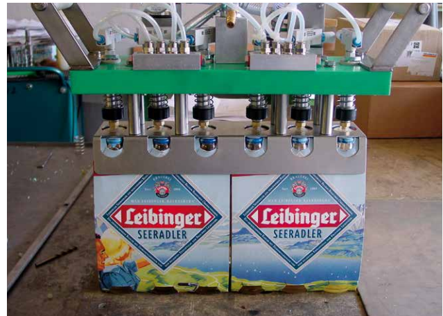
Special manual packing head to move two six pack packages into pin-partitioned crates
