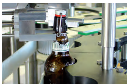
The alignment station lowers onto the closed swing stopper, the alignment flap engages and turns the bottle to the opening position.
