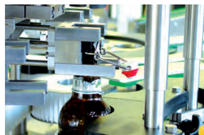
Lifting the swing stopper Escaping liquids or dirt cannot harm the bottle plate located under the bottle.
