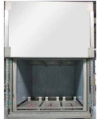
Automatic lift gate
