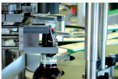
The press-on station opens the swing stopper. The pressure is adjustable, and the sliders are cam-controlled.
