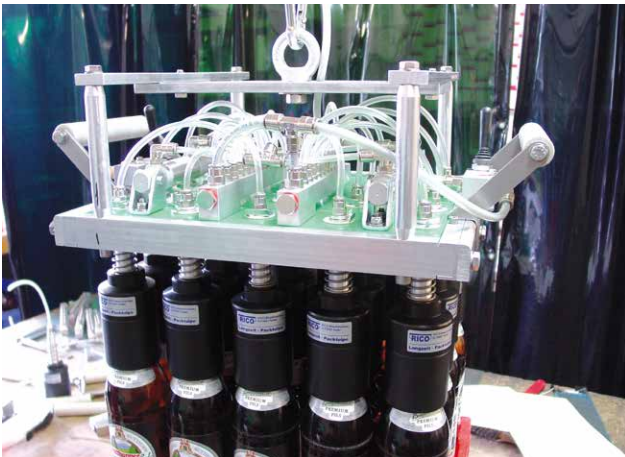
20-piece manual packing head for 0.5 l Euro bottles
