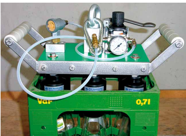
6-piece manual packing head for 0.7 l VdF bottles
